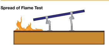
Flame at southern edge of roof is aimed up the roof as a fan blows at 12 mph. The flame cannot spread 6 feet or more in 10 minutes.
