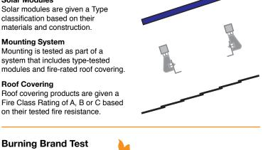
A burning wooden block is placed on module as a fan blows at 12 mph. Flame cannot be seen on underside of roof within 90 minutes.
